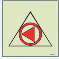
FCS214 Remote control for emergency fire pump or fire pump supplied by the emergency source of power
